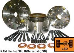
KAM offers a unique solution for a fully adjustable and upgradeable differential assembly (i.e. you can have both full diff locker and LSD combination).
